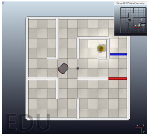
Figure 12. Robot get stuck in a certain position.
