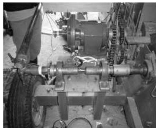
**Gambar 1.** Pengukuran kalibrasi strain - torsi
