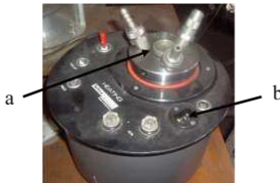
Figure 5 Liquid test cell from Tettex Instruments for dielectric constant and dissipation factor measurements; (a) Thermometer, and (b) heater's terminal.
