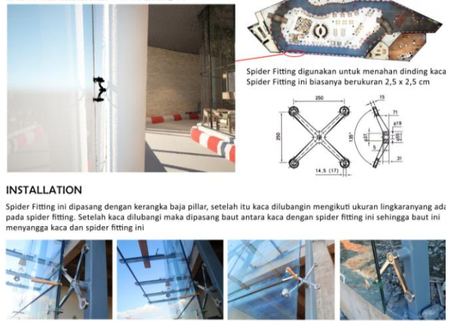
Gambar. 30. Detail Spider Fitting Glass
