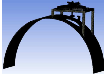
Figure 3 Meshed model of the fixed cutting configuration of the CNC flame processing system.
