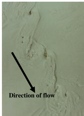
Figure 2 Vortices at the interface between the main channel and floodplain flow, Medicine Hat, Alberta (Tuitoek, D.K., [2]).
