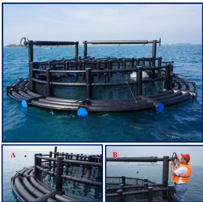
Figure 3. Installation KJABB - IMTA in sea farming region Reef Width , Kpeulauan Thousand ; A. Foot step with rounded bench along the outer circle KJA ; B. Net roller to steer connected by PE rope with a net over
