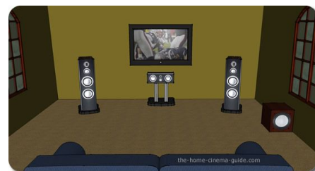
Fig 5. Recommended Front Speaker Placement
