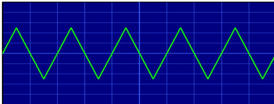
Figure 2. Triangular Wave, Frequency 2500 Hz, Amplitude 10 V.
