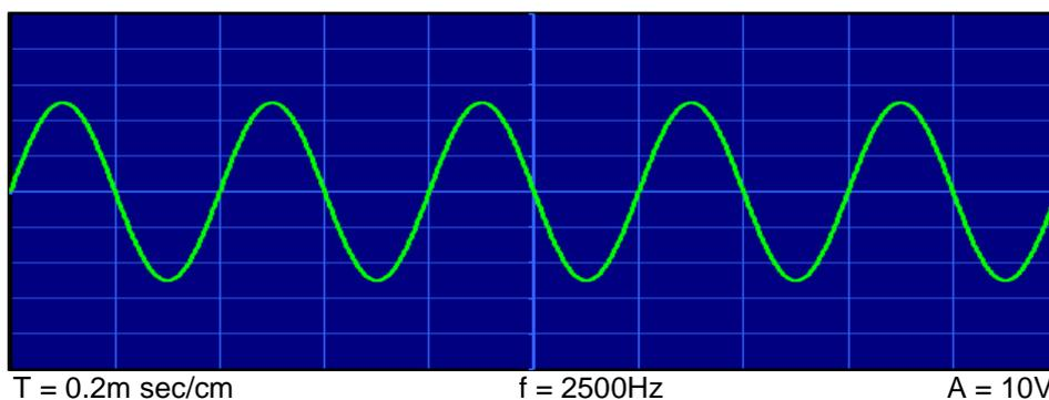
Figure.1 Sine Wave, Frequency 2500 Hz, Amplitude 10 V
