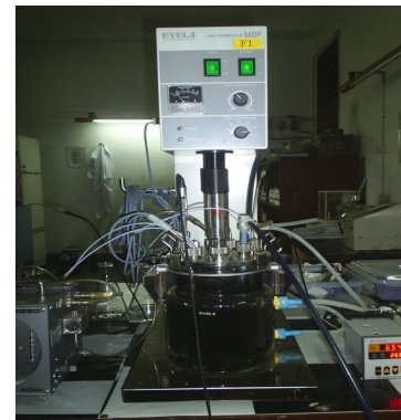
Fig. 1. Two-litre biodigester used for POME fermentation
