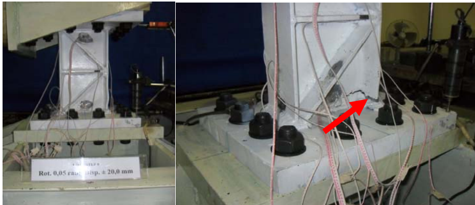
Figure 13 Cracks in the flange of the Specimen I in the top of the welded joints, no buckling occurred in the diagonal stiffener during collapse.
