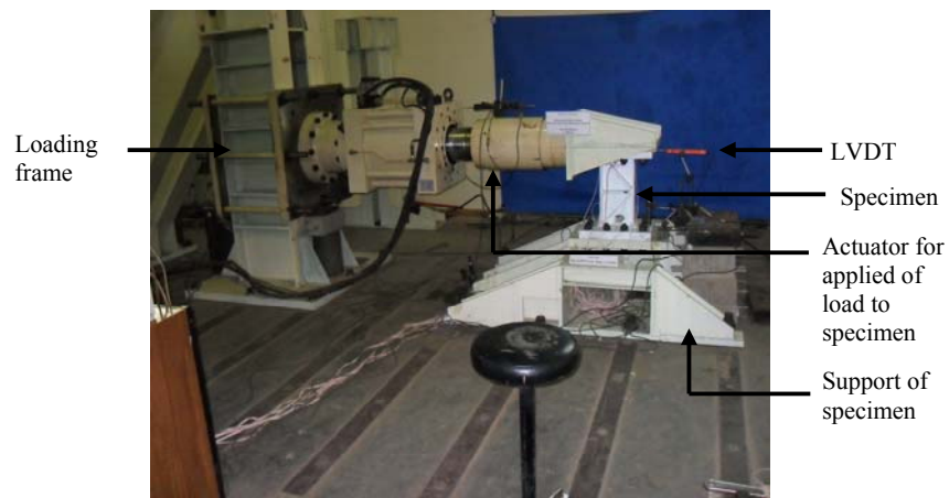
Figure 8 Set up of equipment and specimen of shear link.
