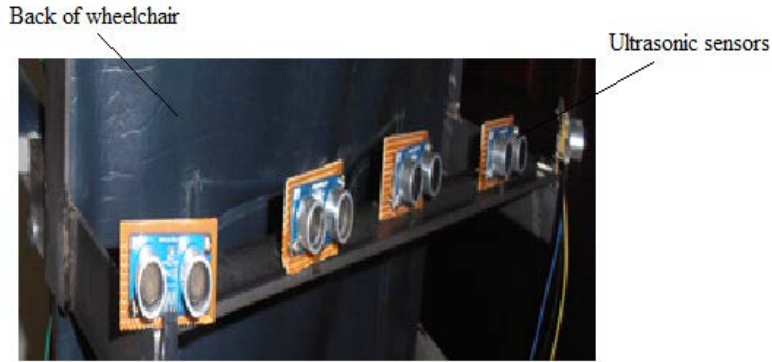
Figure 14 Installation of 5 ultrasonic sensors.
