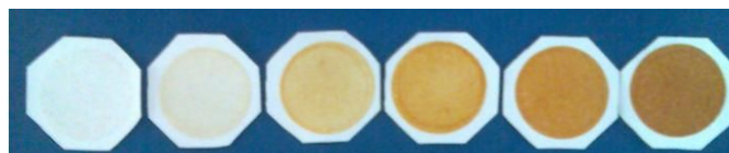
Fig. 11. Sludge of settled SS on the bottom of settling column and the glass-fiber filter that have been filtered the SS at 0 min (before treatment), 10 min, 15 min, 20 min, 25 min and 30 min, respectively.
