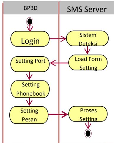
Gambar 11. Activity Diagram Setting Device
