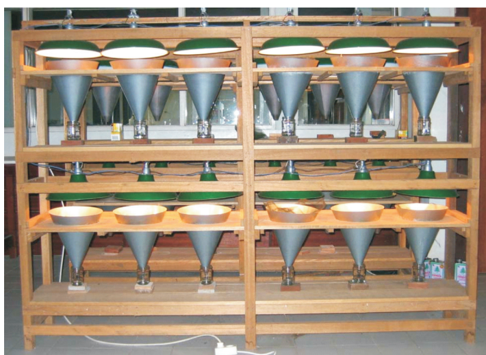
Gambar 1. Alat perangkap tungau Berlese funnel ( Berlese funnel mites trap equipment )
