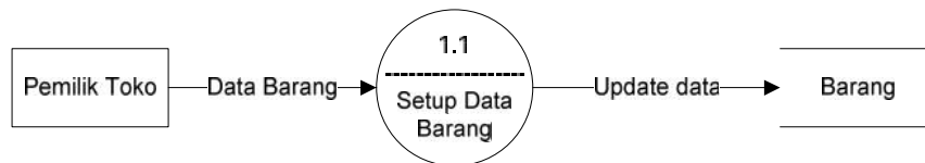
Gambar 3. Data Flow Diagram Setup Barang Level 1
