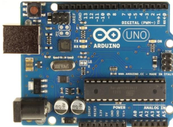
Gambar 1. Microcontroller Arduino Uno
