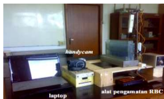
GAMBAR 5. Foto set-up alat pengamatan RBC.
