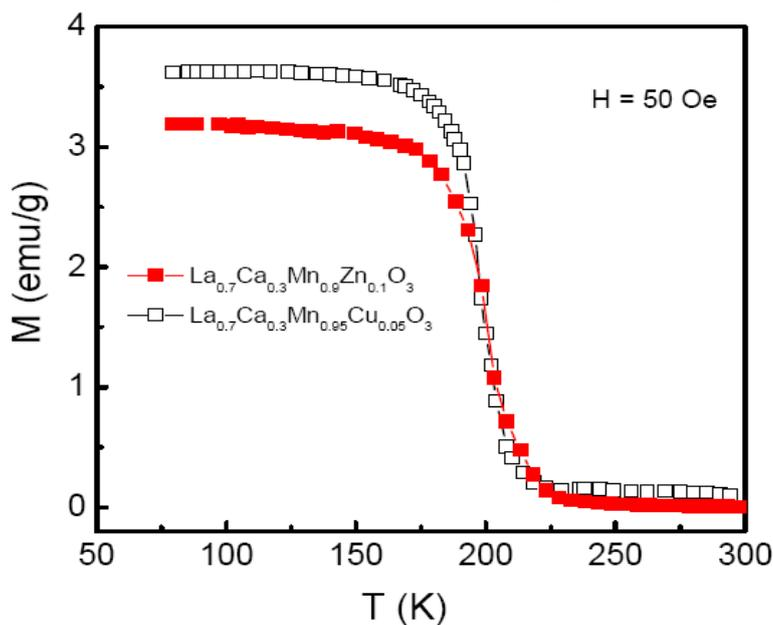
Figure 3. Temperature dependence of the zero-field cooled magnetization for  $\text{La}_{0.7}\text{Ca}_{0.3}\text{Mn}_{0.9}\text{Zn}_{0.1}\text{O}_3$  and  $\text{La}_{0.7}\text{Ca}_{0.3}\text{Mn}_{0.95}\text{Cu}_{0.05}\text{O}_3$  under an applied field of 50 Oe.
