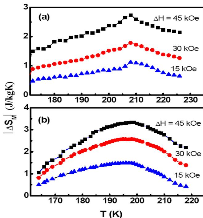
**Figure 4.** Temperature dependences of the magnetic-entropy change for (a)  $\text{La}_{0.7}\text{Ca}_{0.3}\text{Mn}_{0.9}\text{Zn}_{0.1}\text{O}_3$  and (b)  $\text{La}_{0.7}\text{Ca}_{0.3}\text{Mn}_{0.95}\text{Cu}_{0.05}\text{O}_3$  under various applied fields of 15, 30, and 45 kOe.
