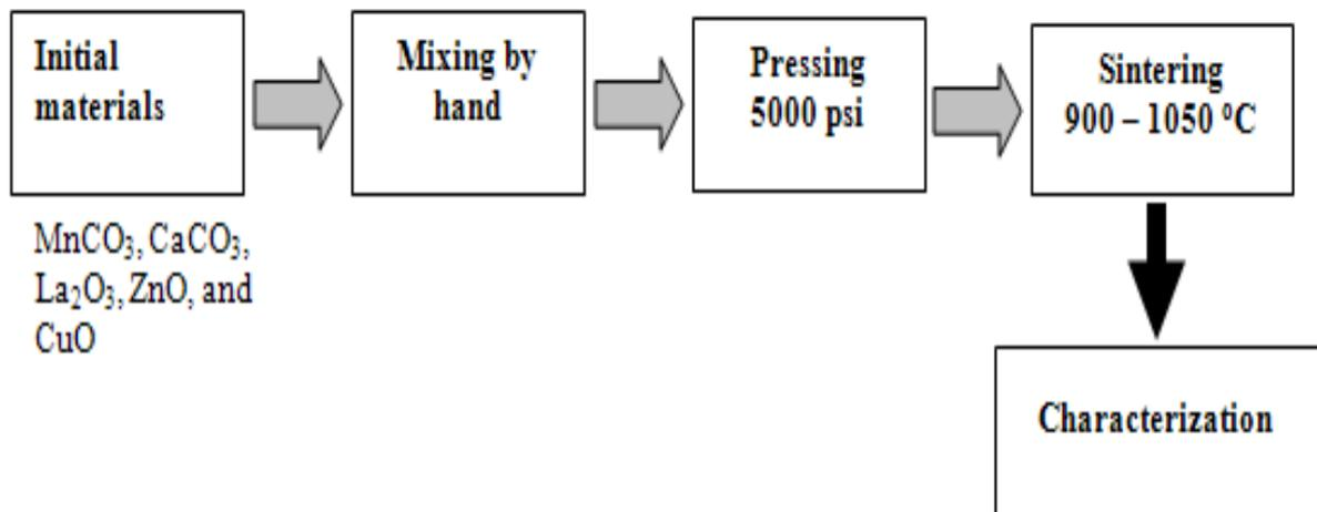
Figure 1. Diagram shows preparation of  $\text{La}_{0.7}\text{Ca}_{0.3}\text{Mn}_{1-x}(\text{Zn,Cu})_x\text{O}_3$  bulks.
