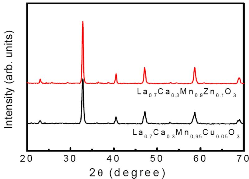
Figure 2. XRD patterns of  $\text{La}_{0.7}\text{Ca}_{0.3}\text{Mn}_{0.9}\text{Zn}_{0.1}\text{O}_3$  and  $\text{La}_{0.7}\text{Ca}_{0.3}\text{Mn}_{0.95}\text{Cu}_{0.05}\text{O}_3$ . The samples are the single phase in an orthorhombic structure (the space group  $Pnma$ ).
