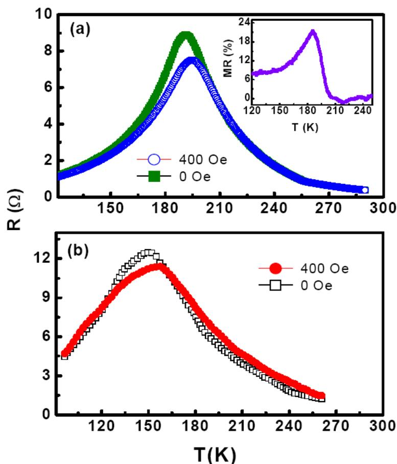
**Figure 6.** Temperature dependences of resistance of (a)  $\text{La}_{0.7}\text{Ca}_{0.3}\text{Mn}_{0.9}\text{Zn}_{0.1}\text{O}_3$  and (b)  $\text{La}_{0.7}\text{Ca}_{0.3}\text{Mn}_{0.95}\text{Cu}_{0.05}\text{O}_3$  under applied fields of 0 Oe and 400 Oe. The inset in (a) shows MR of  $\text{La}_{0.7}\text{Ca}_{0.3}\text{Mn}_{0.9}\text{Zn}_{0.1}\text{O}_3$ .
