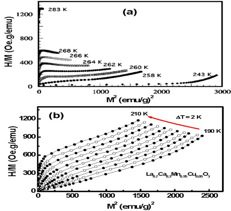
Figure 5.  $H/M$  versus  $M^2$  plots of the isotherms for (a)  $\text{La}_{0.7}\text{Ca}_{0.3}\text{MnO}_3$  (after Mira *et al.* [4]), and (b)  $\text{La}_{0.7}\text{Ca}_{0.3}\text{Mn}_{0.95}\text{Cu}_{0.05}\text{O}_3$ . While the negative slope can be found in (a)  $\text{La}_{0.7}\text{Ca}_{0.3}\text{MnO}_3$  at some temperatures, only the positive slope is found in (b)  $\text{La}_{0.7}\text{Ca}_{0.3}\text{Mn}_{0.95}\text{Cu}_{0.05}\text{O}_3$ .
