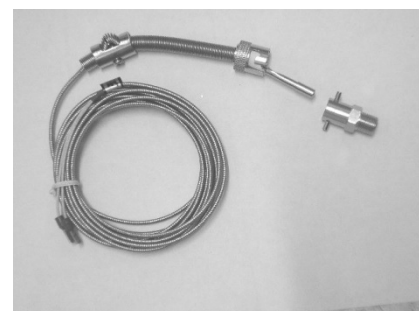
Gambar 7. Sensor suhu Thermokouple tipe-k.
