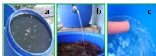
Figure 9. Wastewater collected from the WWTP outlet (a), wastewater condition after passing through the filter at the first drum (b), and the second drum (c)
