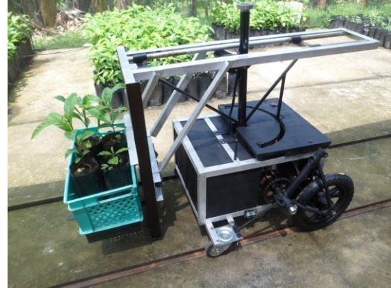
Figure 10. The RC railed robot is transferring polybags.
