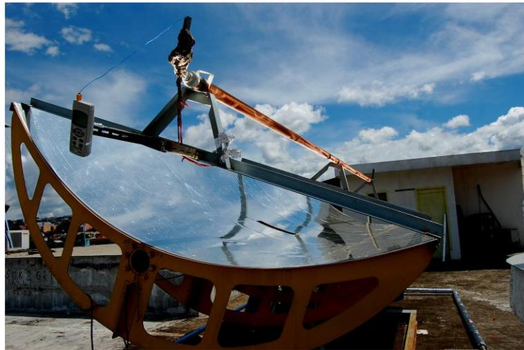
Gambar 2. Prototipe *parabolic trough solar collector*.
