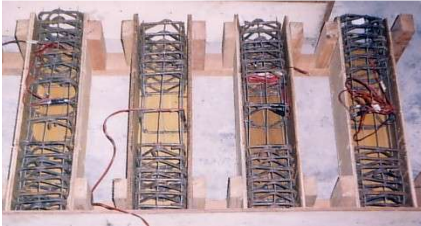
Figure 3 Typical reinforcement cages for confined concrete.
