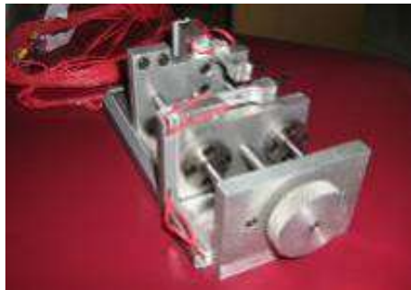
Figure 5 Experimental apparatus for measuring force and moment of a retraction spring [10].
