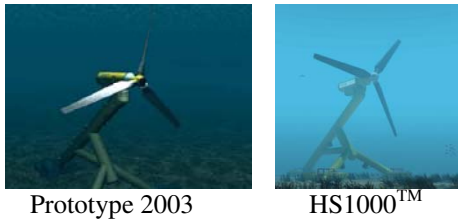
Figure 4. Hammerfest Strom prototypes [4].
