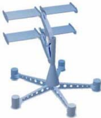
Figure 10. Reciprocating wing turbine prototype [23].
