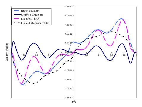
Figure 2 Radial flow velocity distribution for fluid flow through a packed bed.
