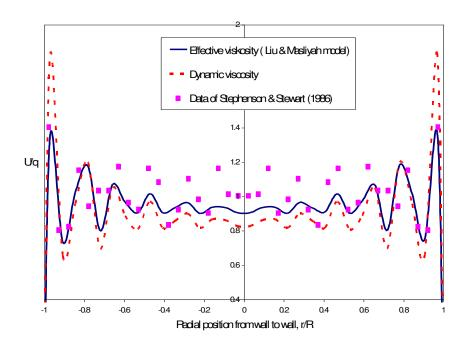
**Figure 4** Influence of effective viscosity to axial velocity profile with high tube to particle diameter ratio (D/d<sub>p</sub>=10.7).
