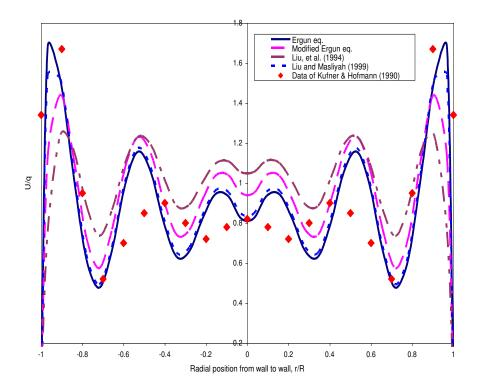
Figure 1 Axial flow velocity distribution for flow through a packed bed.
