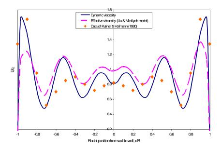
**Figure 3** Influence of effective viscosity to axial velocity profile with low tube to particle diameter ratio  $(D/d_p=4.44)$ .
