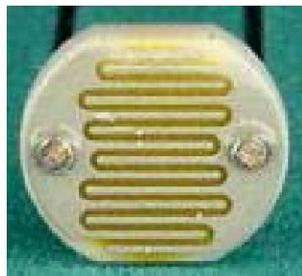
Gambar 1. LDR (Light Dependent Resistor)
