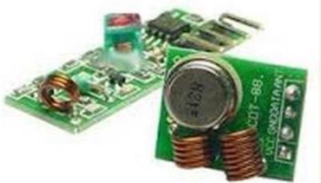
Gambar 3. RF Module Board 433 MHz
