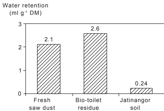
Fig. 4. Water retention of bio-toilet residue and soil.
