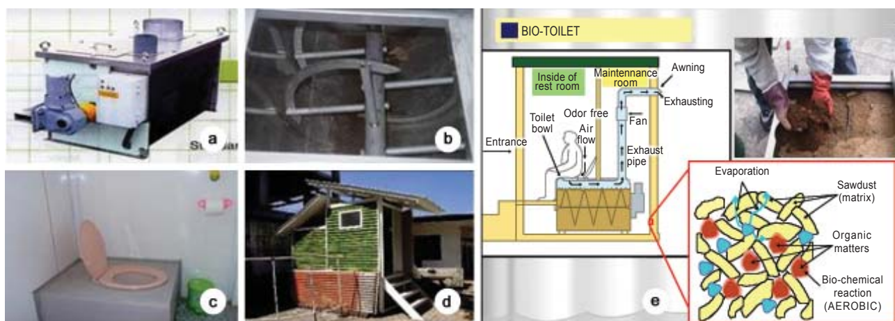
Fig. 1. Bio-toilet type S-50 of Seiwa Denko Co. Ltd. Japan constructed at a private school: (a) bio-toilet chamber, (b) mixer, (c) closet, (d) room of bio-toilet, and (e) schematic diagram of bio-toilet system.
