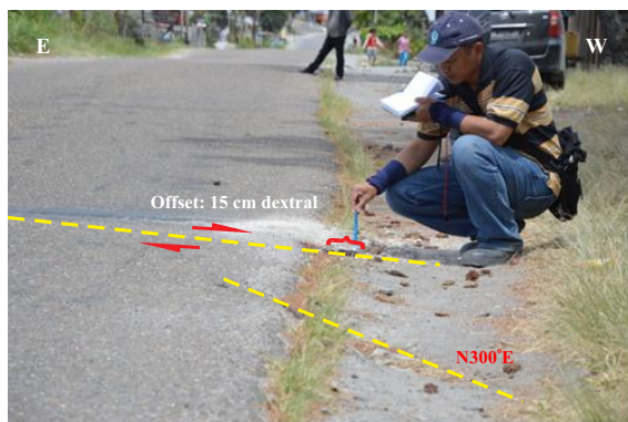
Figure 6. A photograph showing the ground surface rupture at Site 3, Jamur Ujung Village. There are two ruptures with azimuthal trends of 85° and 300°. The inferred dextral offset is 15 cm.
