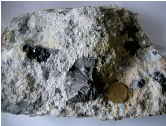
Figure 14. Photograph of marcassite and galena within an altered sericite-quartz vein.
