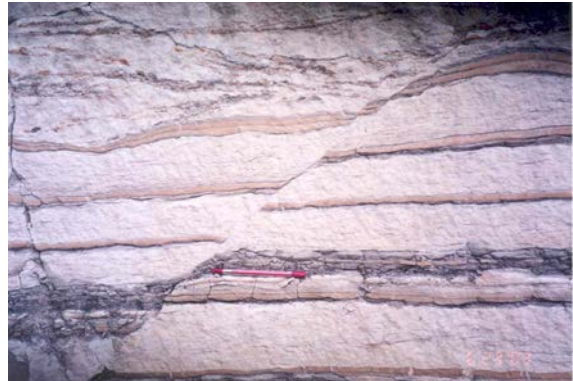
Figure 5. Photograph of sandstone with claystone intercalations at the upper part of the Lati Formation affected by tectonics (micro fault). Binungan traverse 1 (Rachmansjah et al. , 2003).
