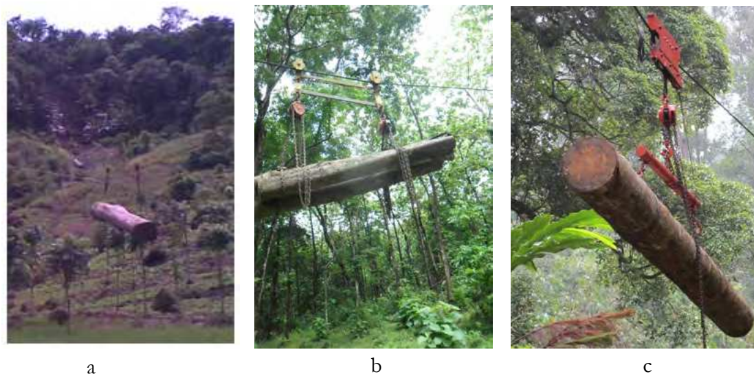
Figure 4. Log extraction by horizontal head position using variation of carriages
