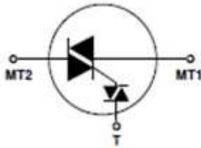
Gambar 4 Internally Triggered TRIAC (IT TRIAC) 3
