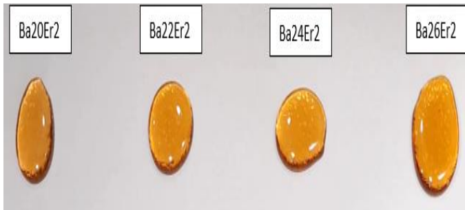
Fig.1. Photographs of the prepared BaO–PbO 2 –B 2 O 3 –Er 2 O 3 glass samples with different BaO content.
