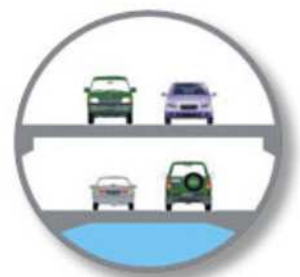
Figure 5b. Typical tunnel cross section
