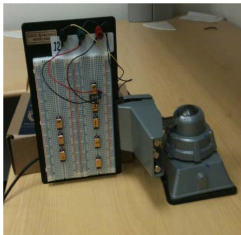
Figure 12. Test set up for Vibration test at 1g
