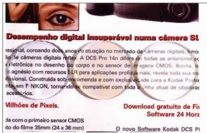
Fig. 4. From left to right: parent glass, glass-ceramic with 97 percent crystallinity and glass-ceramic with 50 percent crystallinity. Grain size is about 20 micrometers.
