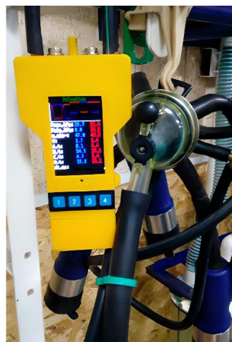
Fig. 5. Milking machine tester v. 2.0
