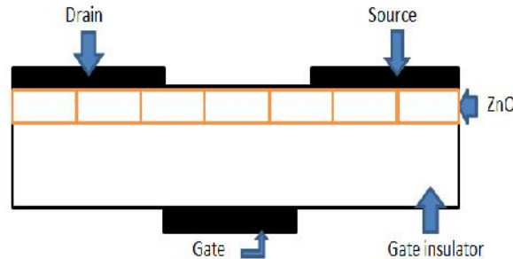
Figure 1. Cross-sectional view of ZnO TFT
