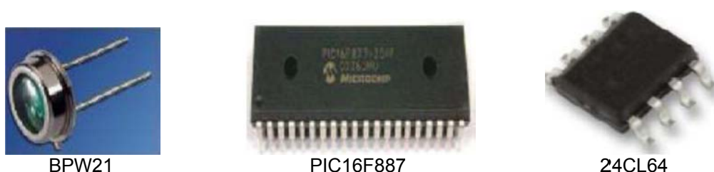
Figure 4. Main components used in this design
