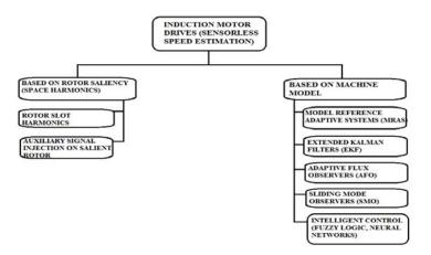
Figure 1. Classification of Speed estimation methods
