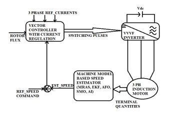
Figure 2. Speed sensorless vector control scheme
