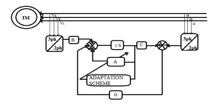
Figure 6. Adaptive Observer scheme for speed estimation [9]
