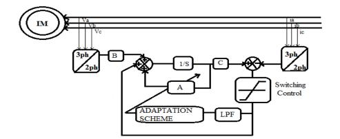
Figure 8. Sliding Mode observer scheme for speed estimation (I.M. Alsofyani et al, 2013)
