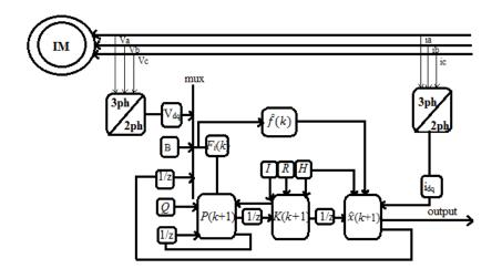
Figure 5. EKF Scheme structure [9]
