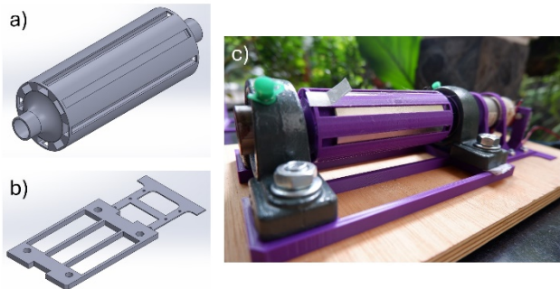
Figure 1. (a) design of the magnetic rotary drum, (b) design of the fixtures, and (c) the photo of the assembled eddy current separator used in this research.
