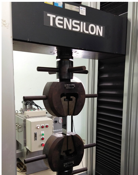
Gambar 2. Proses pengujian lap shear
