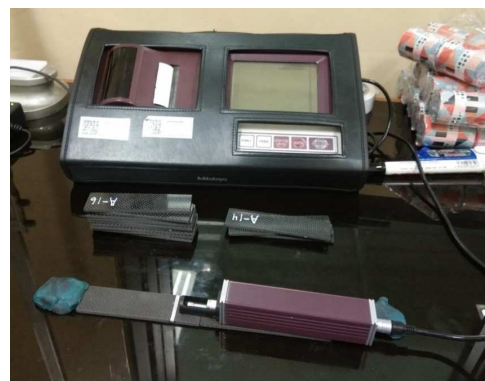
Gambar 1. Pengukuran Surface Roughness
