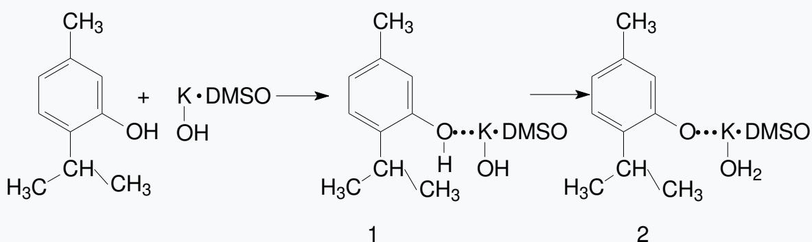
It is known that due to the high mobility of the hydroxyl proton in 5- methyl -2-(1- methylethyl ) phenol , the proton in complex 1 interacts with the hydroxyl group in potassium hydroxide. Complex 1 then passes through a relatively small energy barrier. As a result complex 2 is formed.
