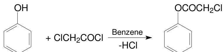
Chloroacetylation reactions were carried out with 5-methyl-2-(1-methylethyl)phenol under different conditions in order to synthesize an individual substance similar to the above and to synthesize substances with biological activity based on it. The method of obtaining 5-methyl-2-(1-methylethyl)phenylchloroacetate with the highest yield was found. The reaction goes according to the following scheme.
