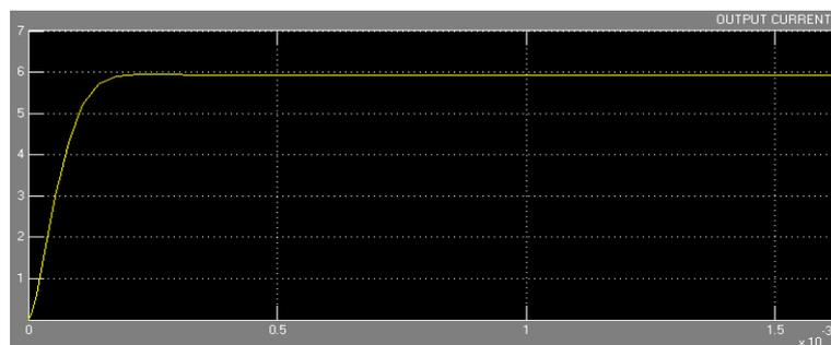
Figure 11. Output Current waveform of Buck Waveform using Sliding Mode Controller
