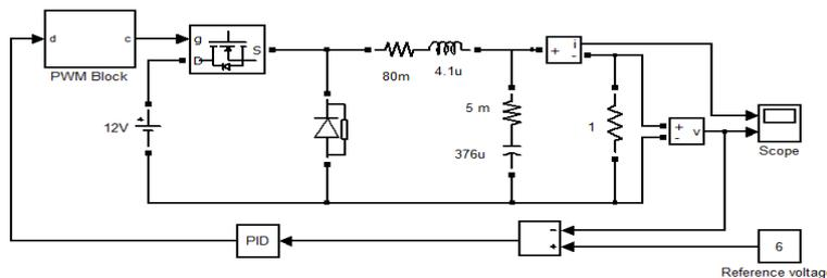
Figure 7. Simulink Model of Buck Converter using PI Controller
