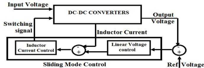
Figure 5. Block Diagram of Sliding Mode Control
