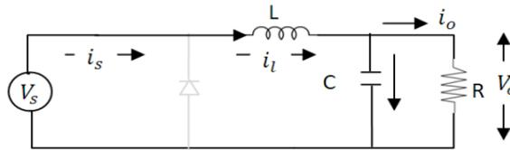
Figure 2. Equivalent circuit during turn ON
