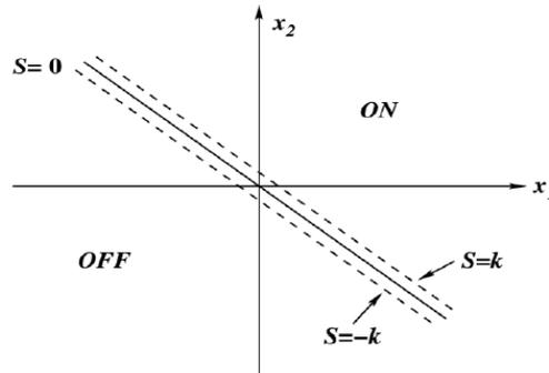
Figure 6. Sliding mode on  $x_1$ - $x_2$  phase plane
