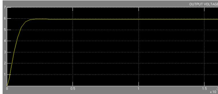
Figure 12. Output Voltage waveform of Buck Waveform using Sliding Mode Controller
