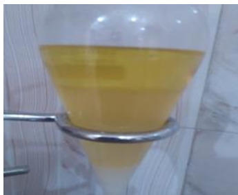
Figure 2. Separating funnel apparatus for phenolics extracted
