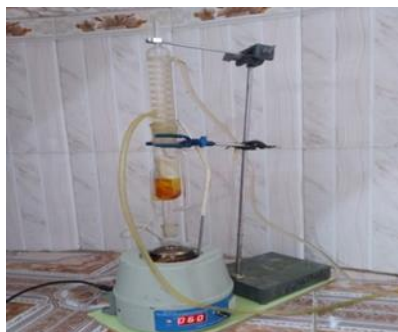
Figure 3. Soxhlet apparatus for terpenoid compounds extracted
