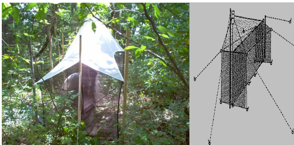
Figure 2. The Malaise trap on the research ground and the scheme of Malaise trap
