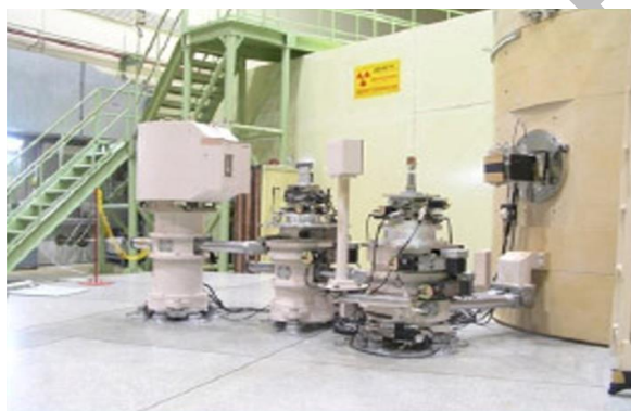
Fig. 1. The neutron triple-axis spectrometer (TAS)
