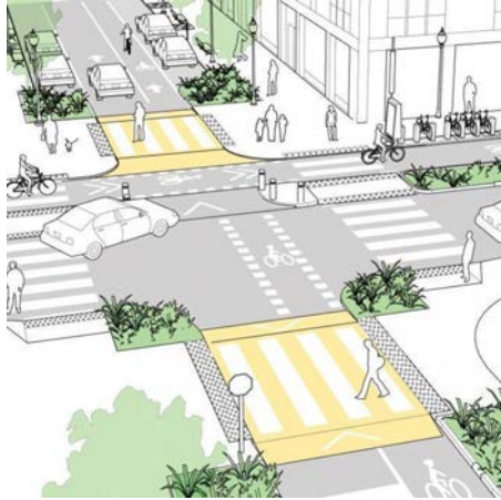
Fig. 6.22 An example of arranging safe pedestrian and bicycle paths at an unregulated intersection [30]
