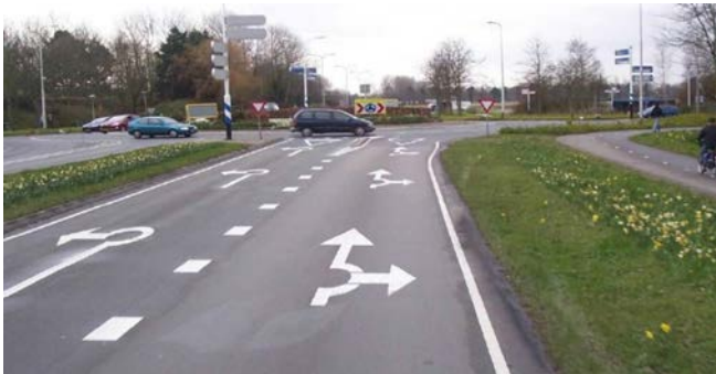
Fig. 6.18 Circular intersection at the same level [26]
